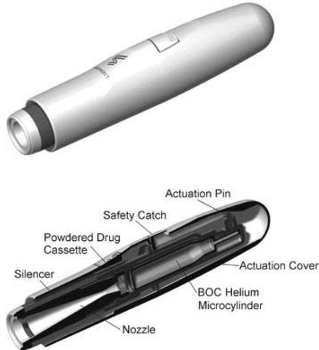
PowderJect Injection Device<sup>189</sup>
